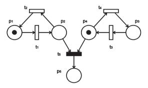
Figure 4. PN that models a test in the system.
