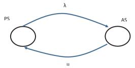
Figure 18. State transitions of intermittent fault.
