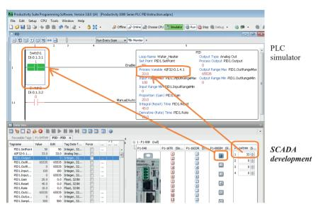
Simultaneously with the development of the PLC program, visualization was also developed using Scada software. Reliance Scada was chosen. Based on the requirements of the operator, the initial version of the visualization was created and according to comments and later experience from the operation, it was modified to the final form.
