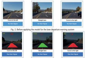
Fig. 3. After applying the model for the lane departure warning system
