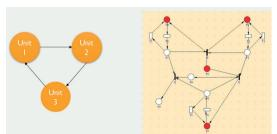
Figure 12. Petri net which models mutual testing in the system after removing two faulty units.
