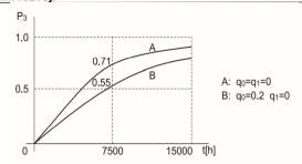
Figure 2. Probability of system failure, P<sub>3</sub>(t).
