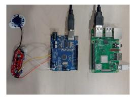
Figure 2: Myoware Muscle sensor, Arduino Uno and Raspberry Pi
