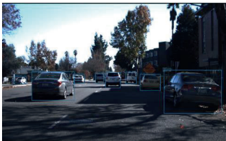
Fig.3.Vehicle Recognition and Tracking from Front Face Monocular Camera
